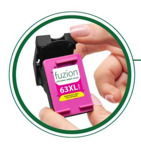
**Step 1:** Remove the plastic protective cap from the ink cartridge.
