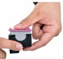
Take out the cover of new cartridge and reassemble the reusable print head and new cartridge together.
